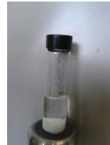
Sample cleaned from interferences, ready for Pb(II) determination using the sensor
