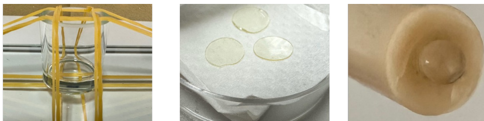
Figure 2. The process of preparation of polymer membrane loaded with ionophor (left and center) and a view of the sensing membrane inserted into a liquid-filled electrode (right)
